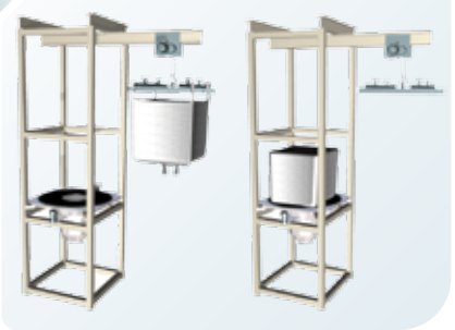
Sisteme big bag yüklenmesi Loading a big bag to the system
