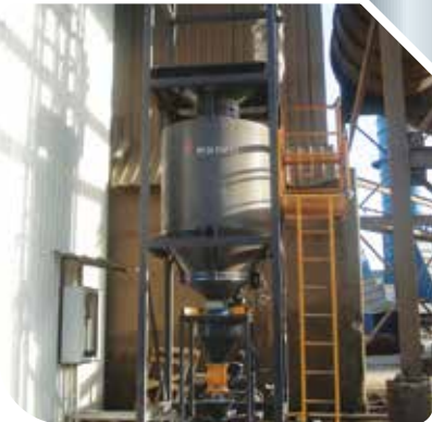
Big bag boşaltma, hammadde depolama, tartım, dozaj ve taşıma sistemi Big bag discharge, storage, weighing, dosing and conveying system
